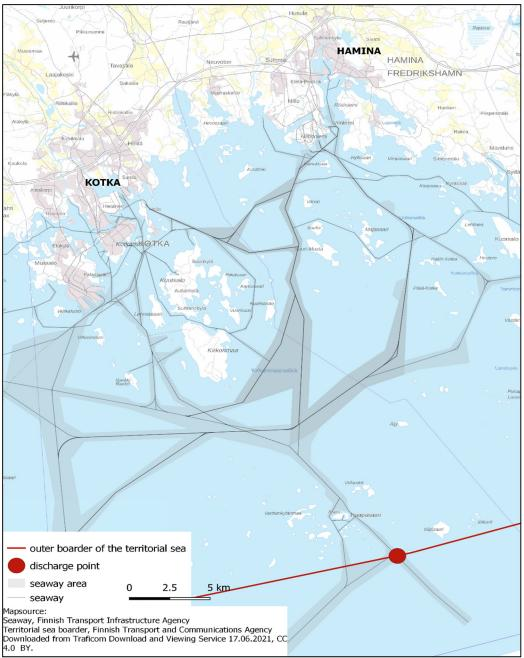
Figure 4. Map of assumed discharge location. According to MARPOL Annex IV, the discharge point for untreated black water should be at least 12 nautical miles from the nearest land.
